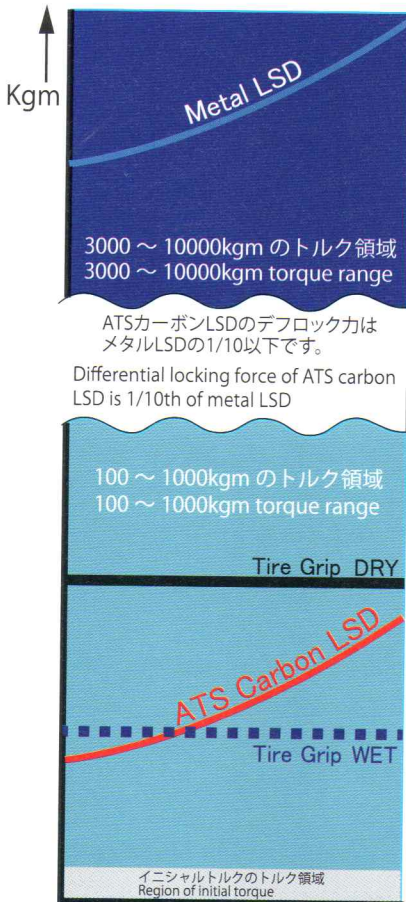
加速旋回中のデフロック力と タイヤグリップ力の相関関係図 Correlation diagram between locking force and tire grip force during acceleration turn
