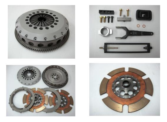
ATS has released newly designed metal twin clutch for Honda S2000 and Acura NSX. This performance clutch can enhance the driving pleasure for the tuned S2000 and NSX. It is offered with two clamping rate—1,100kg and 1,350kg. The clutch can handle 450 hp with the 1,100kg clamping rate and 550 - 600 hp with the 1,350kg clamping rate. Perfect for the turbo or super charged S2000 and NSX.
